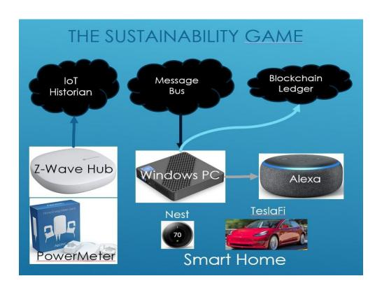
The game system consists of four separate but integrated subsystems; 1) power monitoring, 2) player software agent, 3) data distribution and 4) distributed ledger. Each subsystem was designed to be independent, scalable, extensible and replaceable to allow the system to grow and adapt to a variety of different energy environments.
